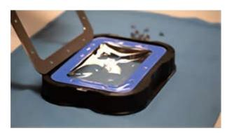
4. Remove the membrane and the gasket from the frame. Discard the old membrane and the gasket in accordance with local laws and regulations.
