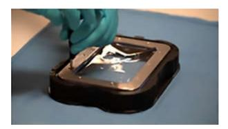
3. Gently lift upward on the resin tray clamp to remove it from the frame.
