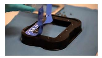
5. Clean the Resin Tray frame and Clamp with IPA. Allow for items to dry thoroughly.
