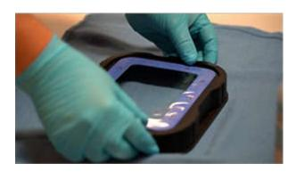
7. Affix the new membrane to the gasket. Make sure to align the holes in the membrane to those in the gasket and in the frame.
